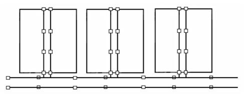
c. "Double Comb Type" layout is an expansion of the "Comb Type" which is recommended for the use in large scale process complexes where five to ten process Units are to be arranged. This layout as shown below in Fig. 3, can be conveniently utilized.
