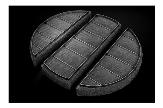
Through careful choice of wire diameter, knitted mesh mist eliminators with extremely high free volumes (typically 98-99%) along with very high removal efficiencies and low pressure drop.
