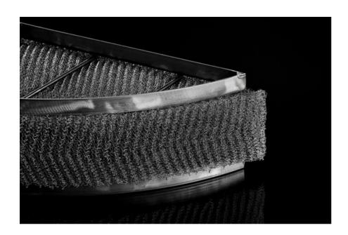
Demister Pads can also be manufactured using plastics for highly corrosive environments.
