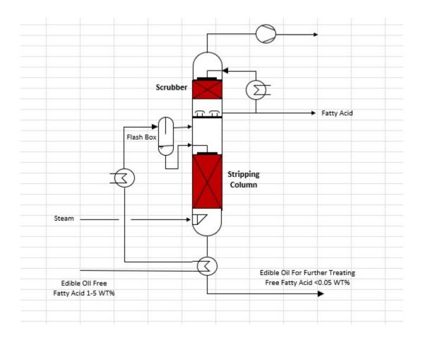
For a single column the top section is called the scrubbing section. The scrubbing section can be one to three beds. The scrubbing section is typically structured packing of KLM 250X EC style. The EC (Enhanced Capacity) is 2<sup>nd</sup> Generation Structured Packing.
