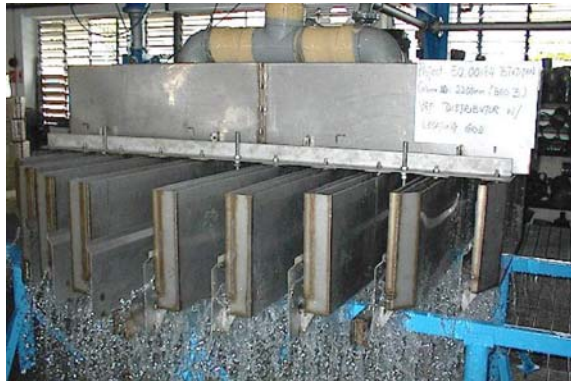
Picture of dual compartment distributor being tested at Sulzer Test Rig in Singapore
