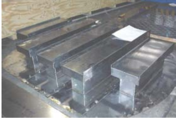
Picture of new Chimney Tray
