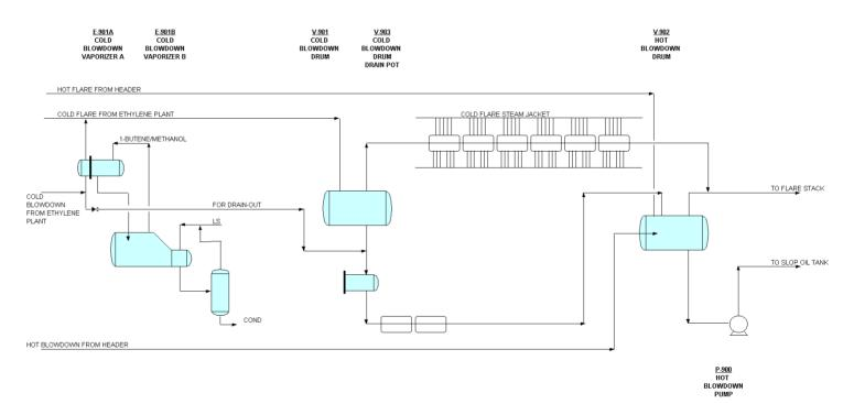
A. Warm Gases / Liquids with KO Drum - Named Hot Blow Down
