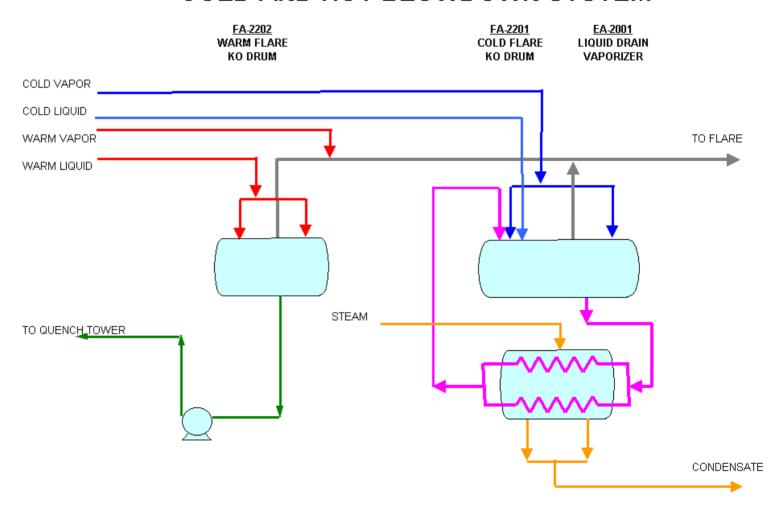
A. Warm Gases / Liquids with KO Drum - Named Wet Or Warm Flare System
