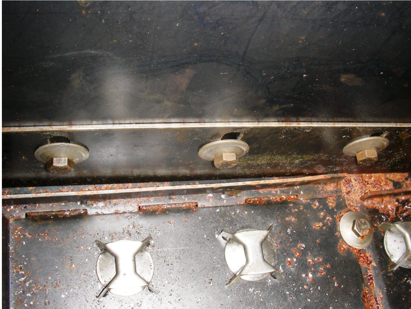
Incorrect Inlet Weir Clearance
