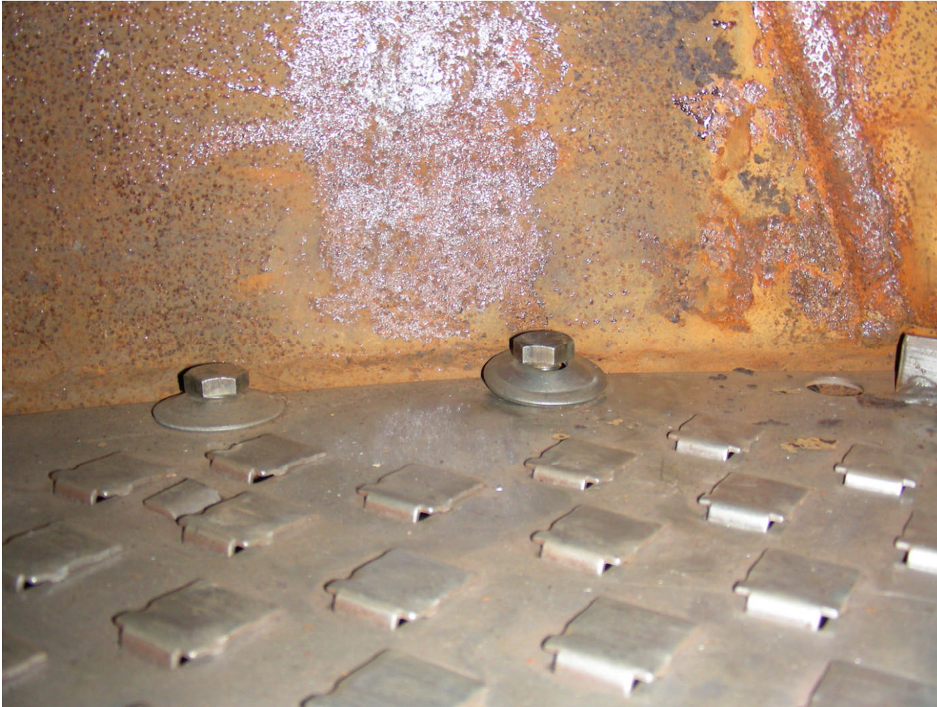
Nuts and Bolts not installed correctly
