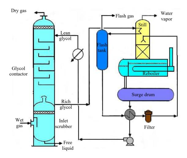
Figure 1: Process flow diagram of glycol dehydration unit
