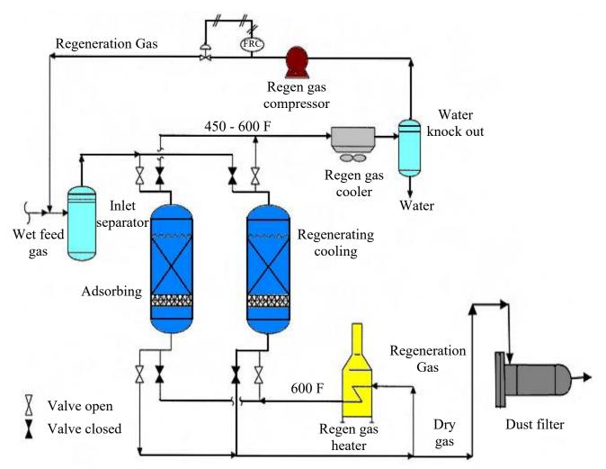
Figure 2: Example Solid Desiccant Dehydrator Twin Tower System
