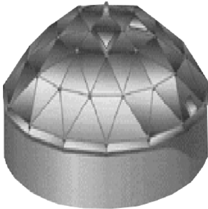
Figure 7: Dome External Floating Roof
