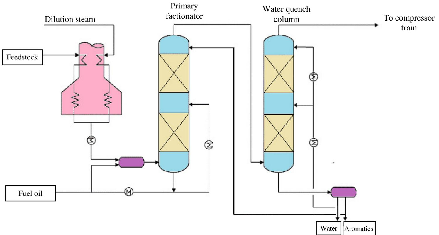
Figure 4: Flow Schematic of Typical Ethylene Quench System
