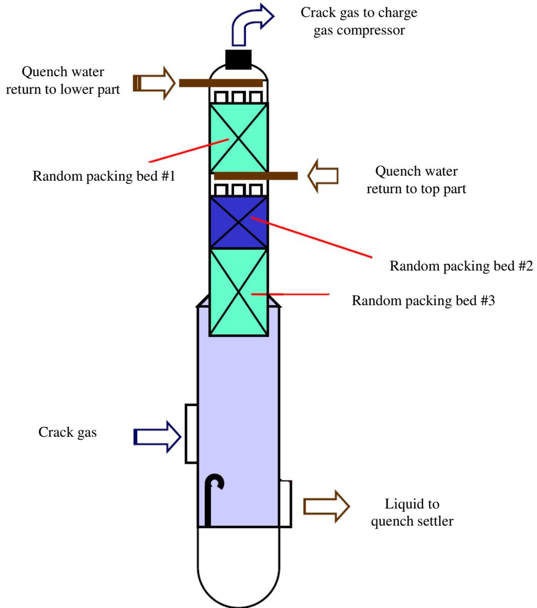
Figure 6: Quench Water Assembly
