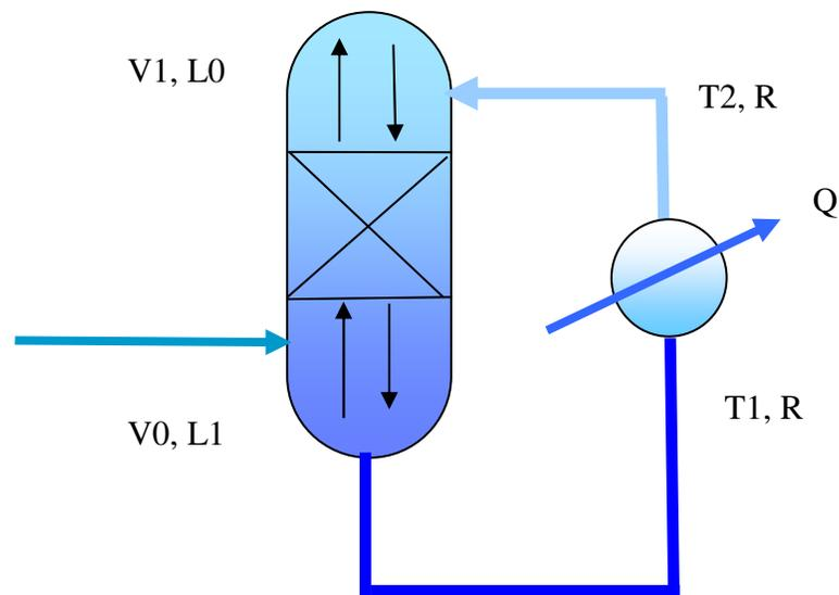
Figure 7: Example of a Typical Pump Around Section.
