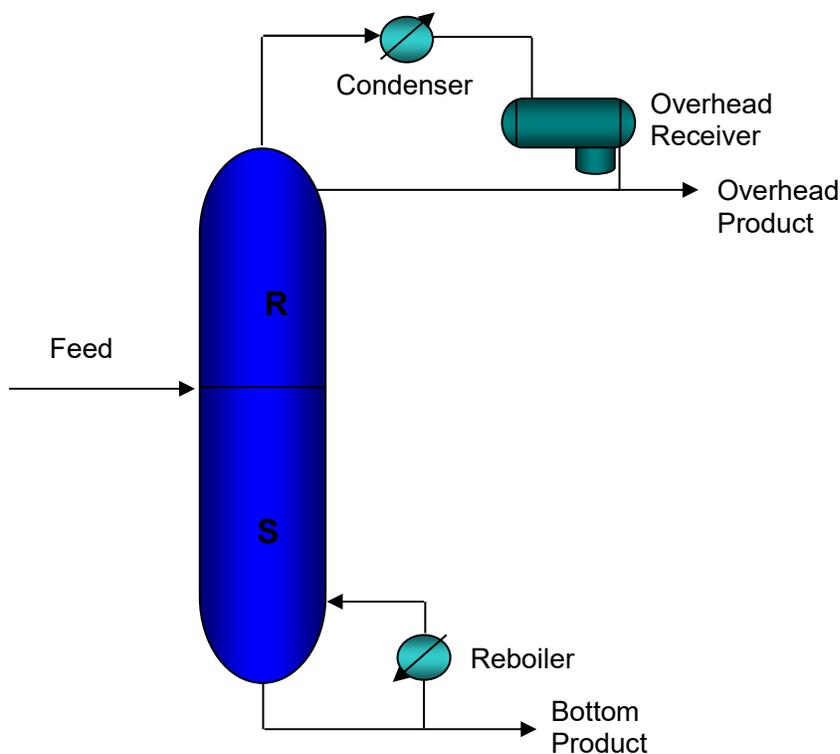
Figure 5: Schematic Diagram of Distillation Column/ Fractionator.
