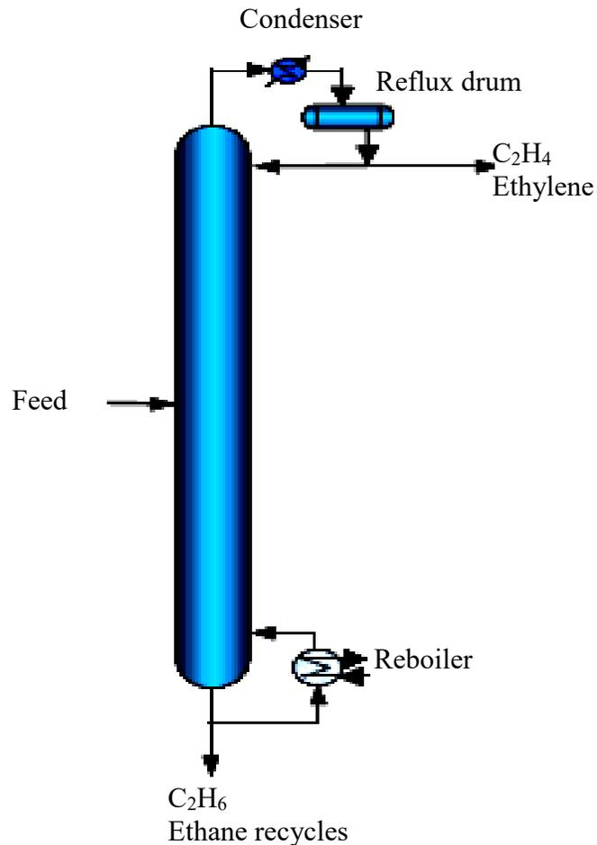
Figure 2: High pressure C2 splitter
