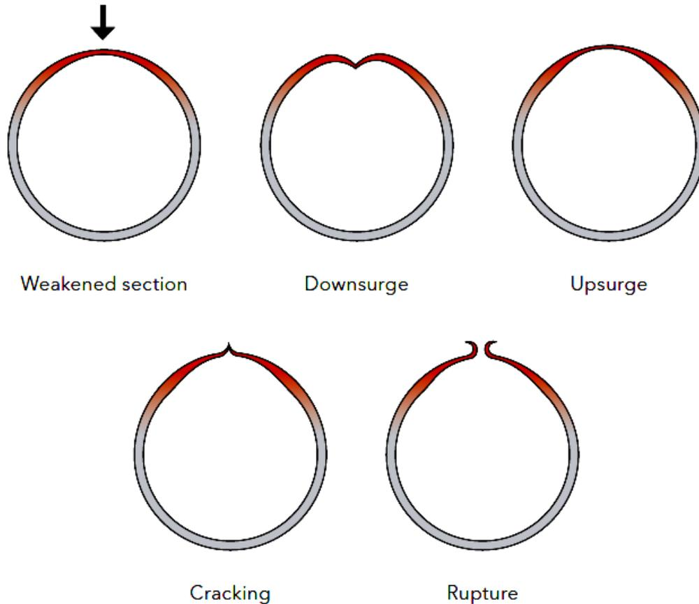
Figure 5: Different effects of a weakened section.
