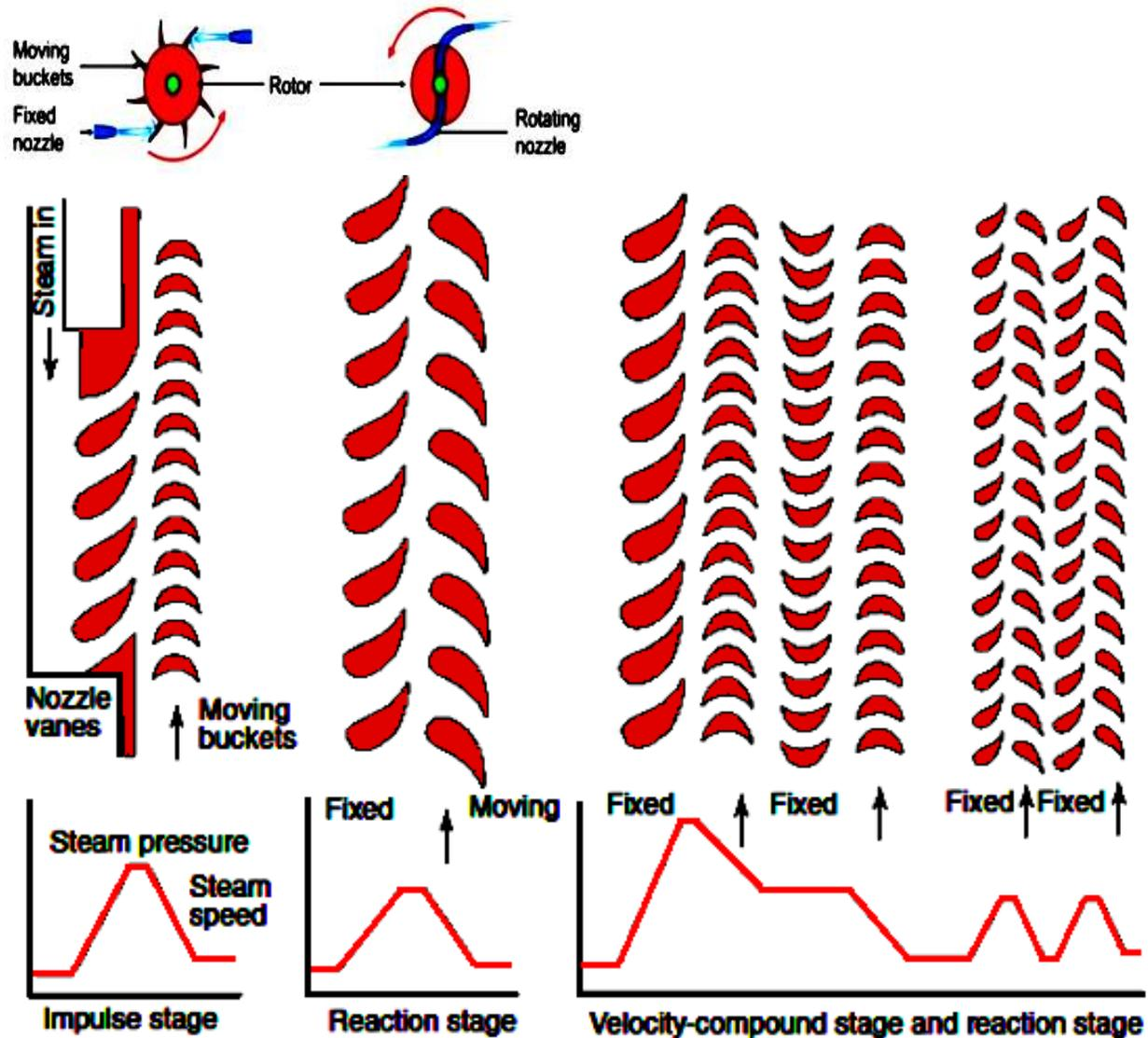
Figure 6: Diagram of simple impulse and reaction turbine stages. (11)
