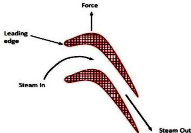
Figure 4: Section of reaction turbine blading
