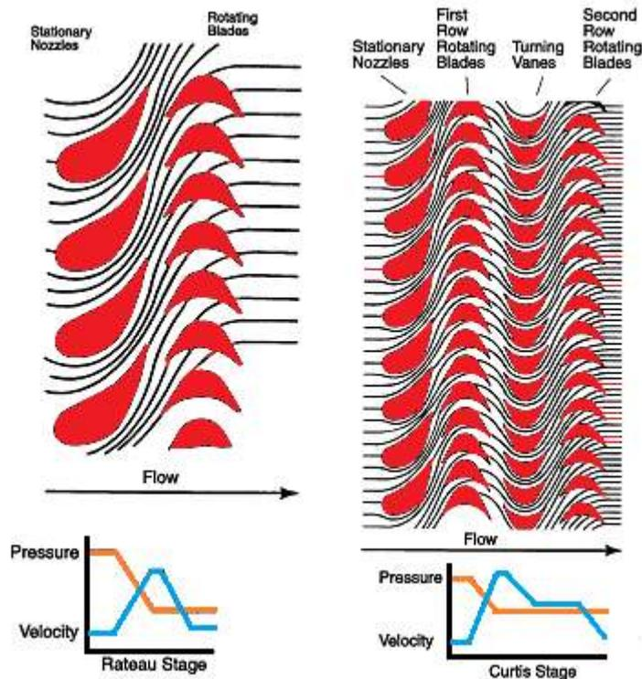
Figure1: Steam turbine blades arrangement
