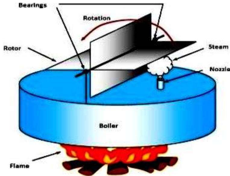
Figure 3: Principle of impulse turbine
