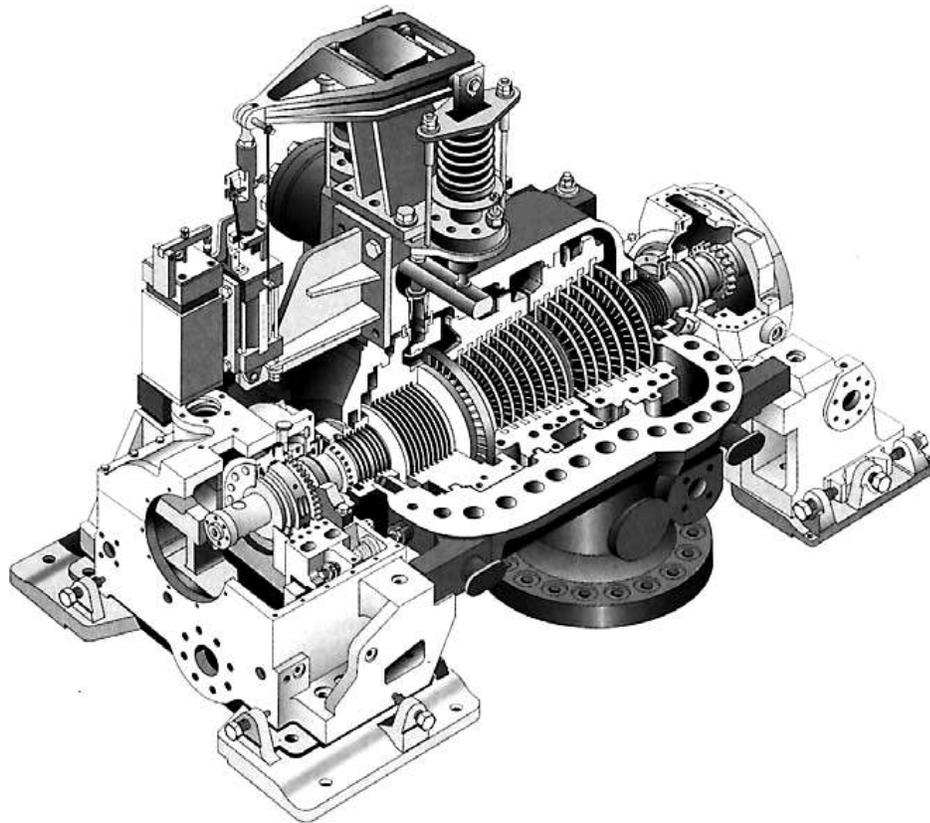
Figure 9: Backpressure steam turbine for approximately 28-MW output. (12)
