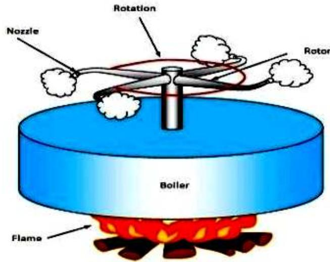
Figure5: Principle of reaction turbine
