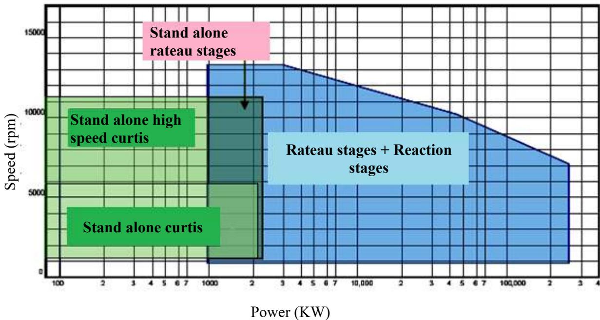
Figure 7: Operating Range of Steam Turbines
