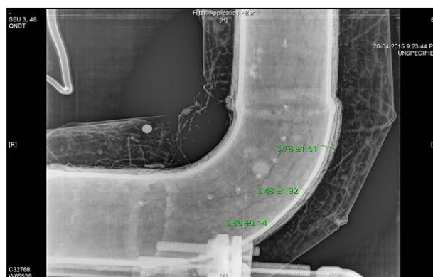
Figure 10 : CR Radiograph Showing Corrosion Deposits.
